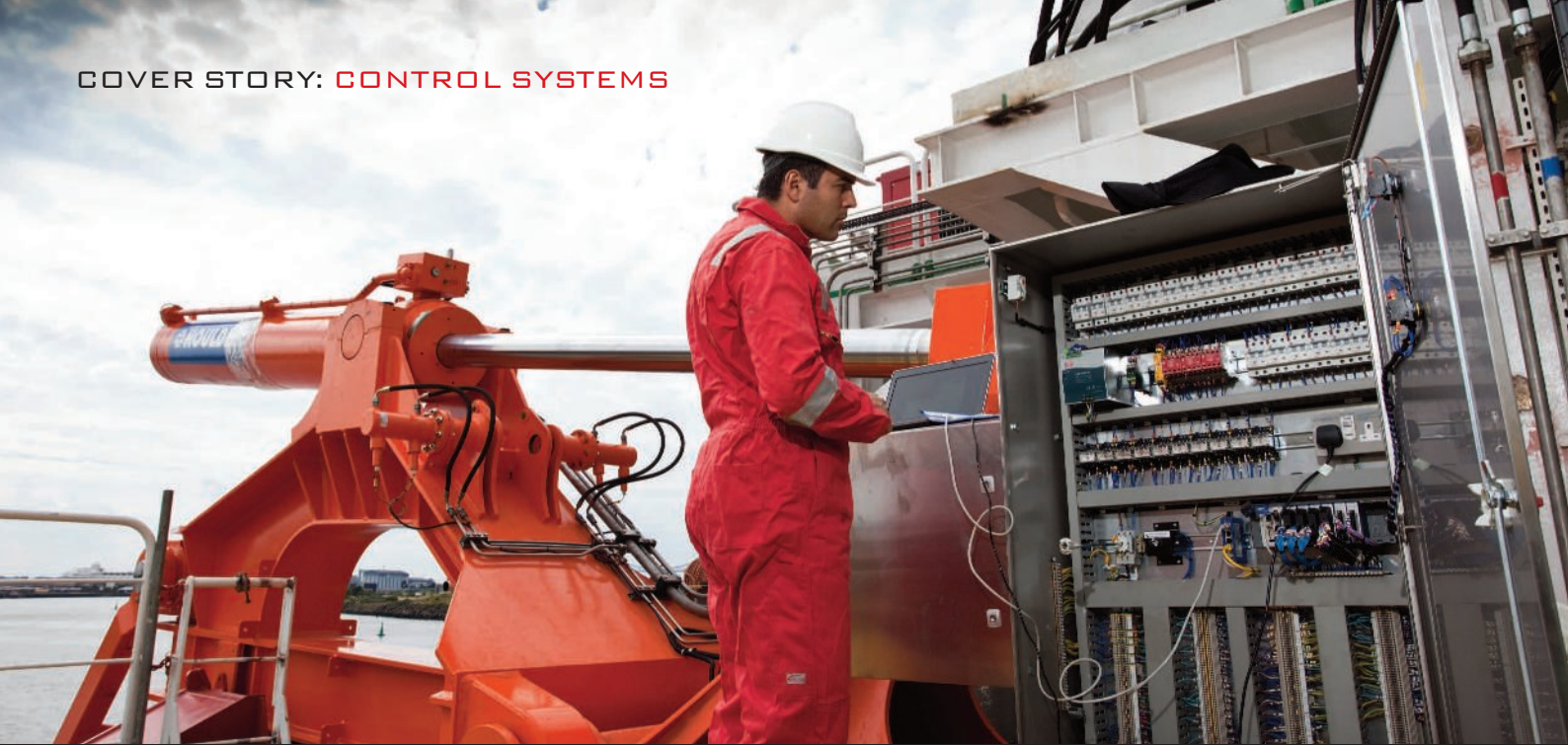
Numerous I/O modules interface with sensors, actuators and the operator (above) to control each hydraulic cylinder precisely (below). Photographs: Chapman Brown Photography
