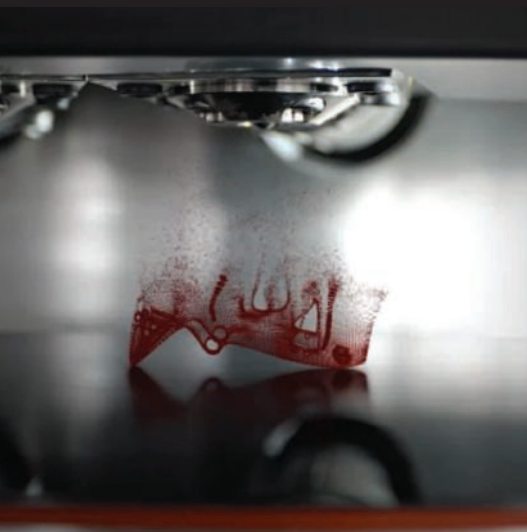
The Arburg Freeformer produces the component without support structures, layer by layer from miniscule droplets, made from standard granulates. The discharge unit with nozzle remains stationary, while the component carrier moves.
