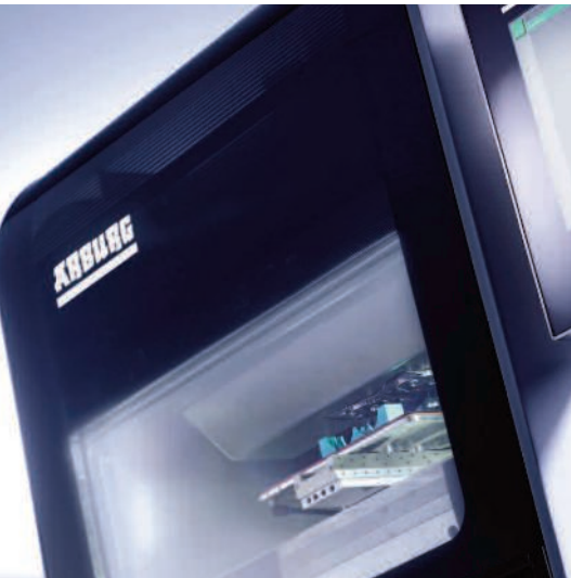
The Arburg Freeformer produces the component without support structures, layer by layer from miniscule droplets, made from standard granulates. The discharge unit with nozzle remains stationary, while the component carrier moves.
